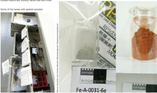
systems are powder samples containing a 1:1-mixture of iron powder (Fe) and fourfold hydrated iron chloride (FeCl2.4 H2O). This will turn into akaganeite - a chloride containing iron mineral which often develops in archaeological iron objects after excavation – when in contact with oxygen and a relative humidity higher than around 15 %.
