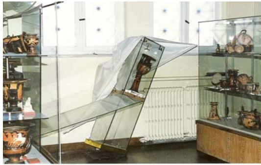
Podany Fig. 4: Protecting individual objects within a collection also involves the design of exhibition and storage furniture (display cases, shelves, etc) that are stable and secure. The collapse or distortion of exhibition cases can cause significant damage to collections, as can be seen in the photograph. (Photograph provided by C. Spyrakos)
