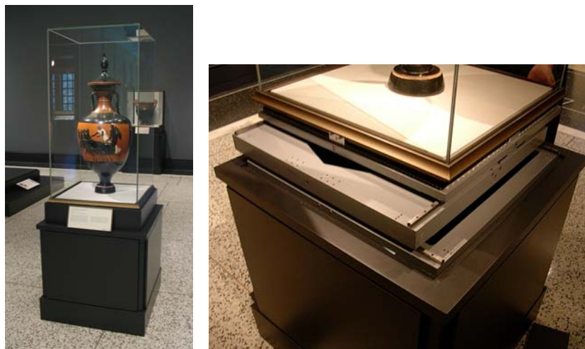
Koumouis Fig. 1: a small scale Getty isolator placed under an exhibition show case at the Getty Museum. On the right, the isolator is shown in a displaced position with the protective panels removed.
