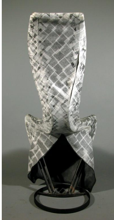
Prototype, S-Chair, Tom Dixon, 1987, consolidation of flaking latex cover with Kozo-paper, photo: Tim Bechthold, copyright: Die Neue Sammlung. The International Design Museum Munich.
