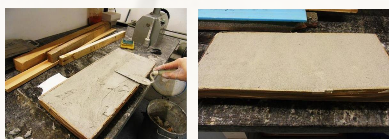
Picture 10: Application of this mortar, in the thickness from 0.2 cm to 3 cm.
