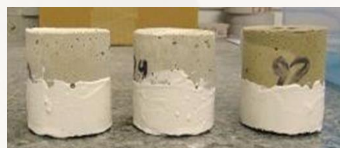
Picture 4: Slag: No presence of efflorescence at 18 %, 36 %, 72 % of activator.
