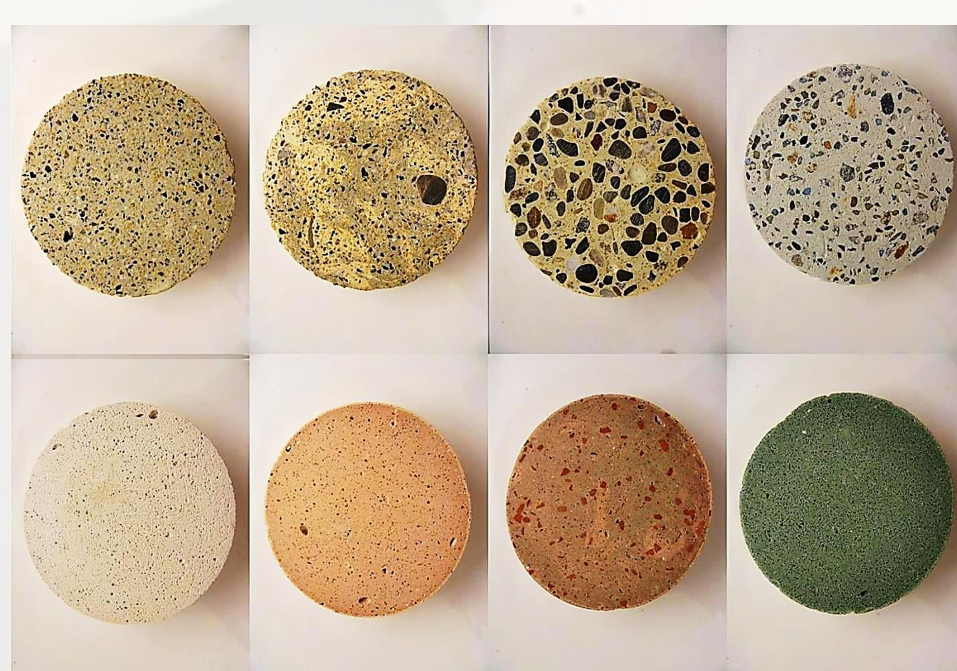
Picture 9: Mortars with different aggregate (grain size and typology), filler and pigments.
