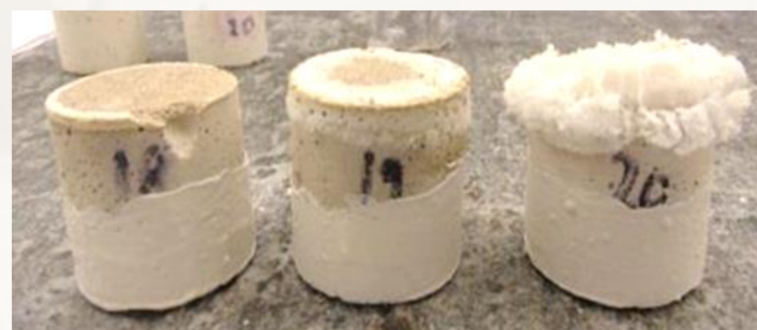
Picture 2: Efflorescence at 18 %, 36 %, 72 % of activator.
