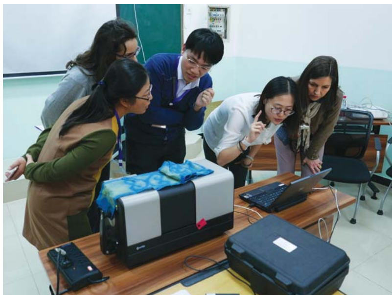
Participants measuring the colours of a piece of faded textile using an integrating sphere spectrophotometer.
