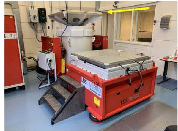
Fig. 2: Vibration testing system. The upper table (arrow) was used for this project.
