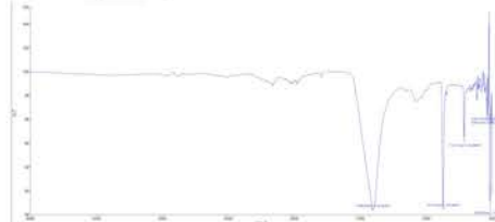
Figure 1. FTIR analyses of calcium carbonate mural painting prototype with three chitosan layers' application, showing only calcite.
