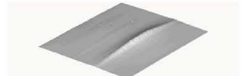
After restoration, 1st nat. freq. 3,6 Hz
