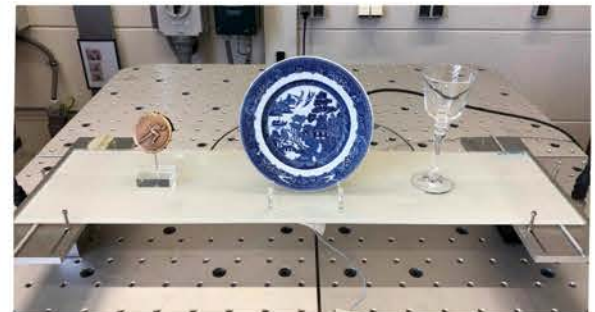
Fig. 3: Glass shelf mounted on vibration table with a three test objects.
