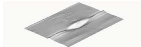
Before restoration, 1st nat. freq. 1,6 Hz
