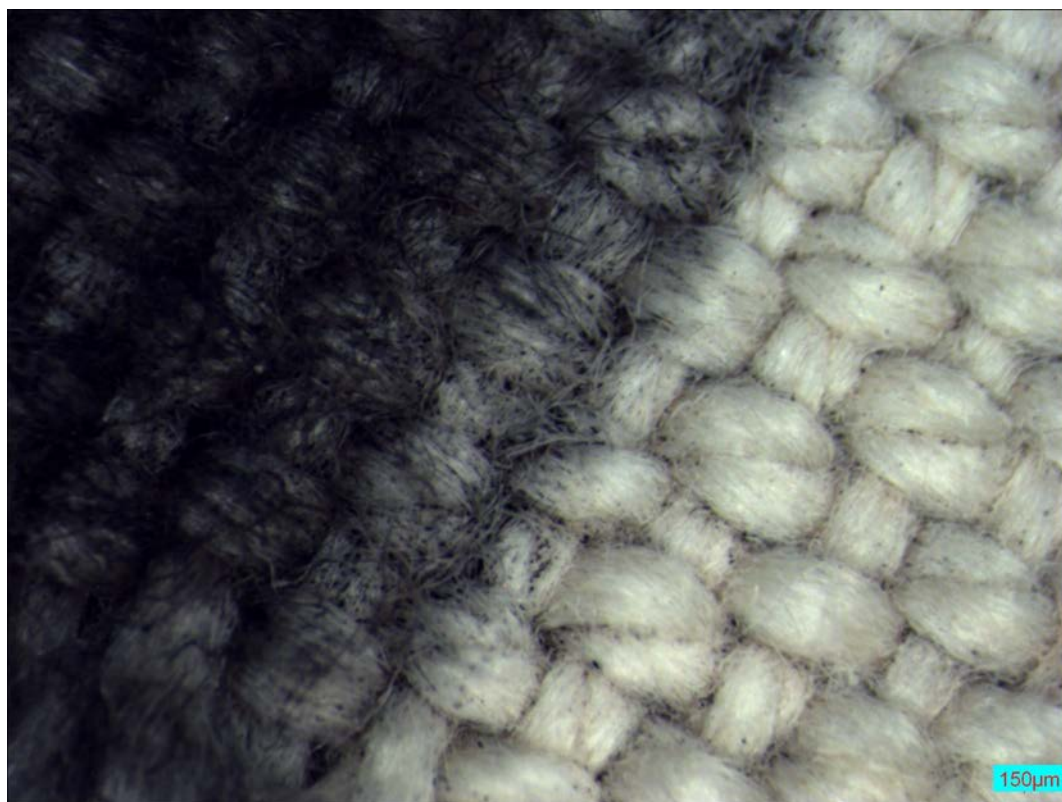
Soot removed from cotton canvas using oxygen atoms under the microscope.
