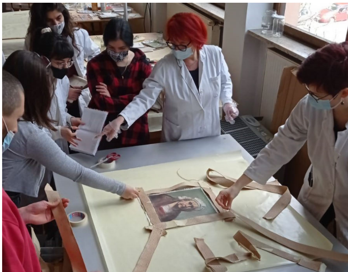
Students and teachers preparing the heat-suction table for lining. Image courtesy of Maja Sučević Miklin
