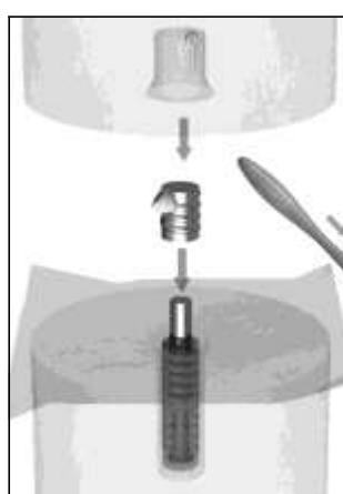
Figure 1a. Inserting the “active” component into the hole in the first piece of marble, using a structural adhesive
