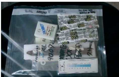
RPSystem®: RP-A® scavenger, oxygen indicator, and datalogger in Escal® bag with iron object.
