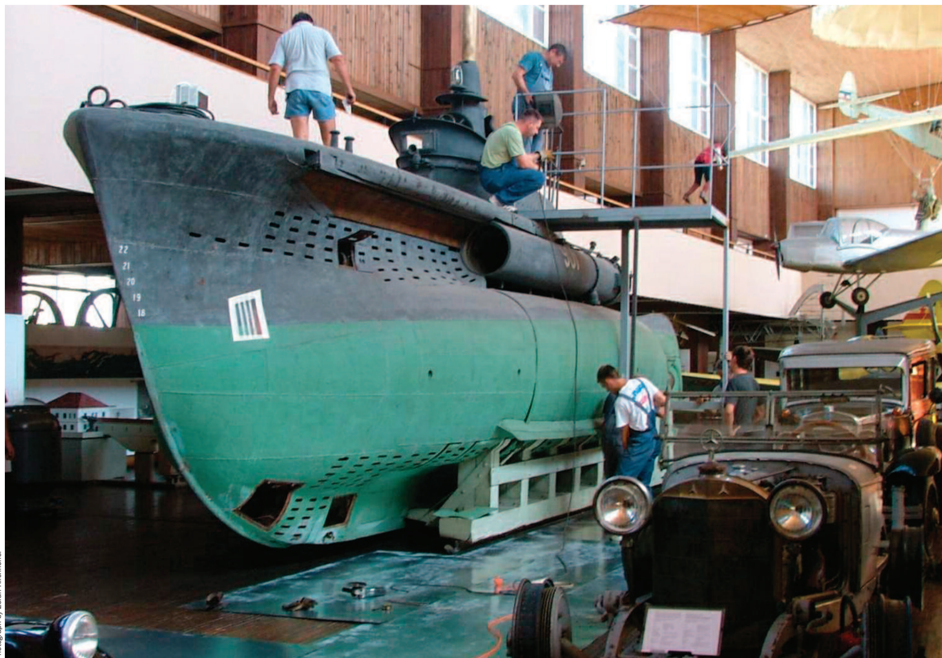
Conservation and restoration works executed on a CB midget submarine No. 20 (CB-20) during 2009.
