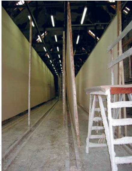
The hand priming facility with a platform where the ground is applied
